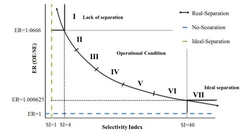
Fig. 6. New upgrading curve based on efficiency ratio (ER) as a function of selectivity index (SI)
